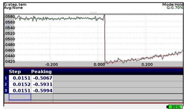
Sensor selection for a step measurement depends entirely on the range of height differences expected. A TS800 sensor with a 0.5" FOV may be necessary for expected ranges of 0.0" to 0.040", while a TS800 sensor with a 1.0" FOV may be required if the expected range is 0.0" to 1.0". A plotted view of the step is not necessary, but it helps to ensure that the feature is centered in sensor FOV. An LG7000 controller will provide this graphical feedback.
