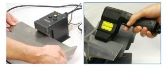
much as 0.350" down to an edge radius of as small as 0.005". Complete data sets, including template matching, blade thickness and radius, are archived along with all of the raw scans and raw sensor images. Available as either handheld portable or benchtop system, a model exists for most any blade inspection application.
