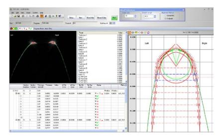
**Programs** – Separate programs can be developed for different blades, specifying different profile nominals and templates and different setback distances for thickness measurements.
