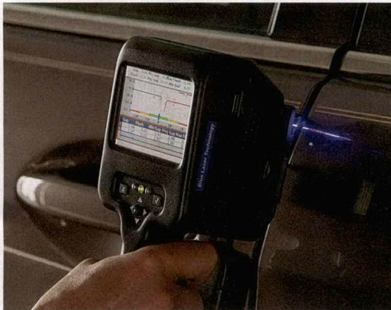
The handheld HS763 sensor measures gaps and flush on translucent, shiny or opaque surfaces around vehicle doors, headlights, taillights, windows and chrome while the car is advancing on a moving assembly line. Photo courtesy Origin Technologies Corp.
